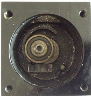
With the end cover removed the extent of the bottom end damage is clear.
