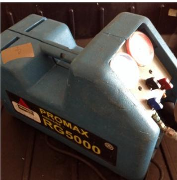
Both dust caps are missing as are several machine screws that secure the casing.
