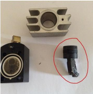
Upon removal of the cylinder head it was apparent that the unit compressor has suffered serious damage.
