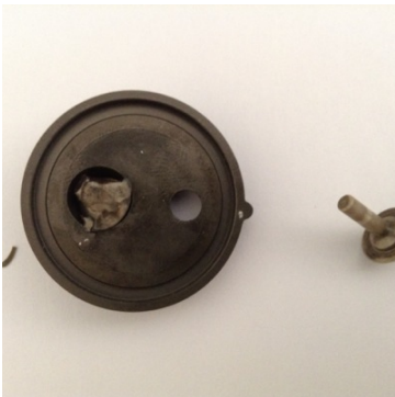
Upon inspection of the valve plate it became apparent that there was significant damage to the suction valve as can be seen in the picture.
